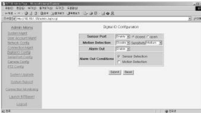
The motion detection is set up for the camera input of the web camera, and the value for its sensitivity has four levels between "Low" and "Very High." In case of "Very High" value, you need to test its sensitivity first, because it may be more likely to trigger false alarms. Refer to the "2.7 Camera Configuration" for the instructions on e-mailing the image of a target camera when an alarm is triggered or motion is detected.
