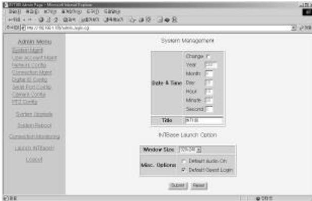
Click System Mgmt to set up System Management and Web Base Launch Option information. The System Management sets the date, time, and system name. The system name will be displayed in the title bar of the web camera base.
